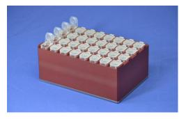
Depending on the type of magnetic beads and the suspension media, volumes up to 1.2 mL can be used. Magnetic beads are collected on the bottom of the tubes, allowing aspiration and transfer of supernatants in depletion protocols. The magnetic separator is designed to fit 32 FlipTubes simultaneously, allowing automated processing for small throughput applications using magnetic beads in centrifuge tubes.
