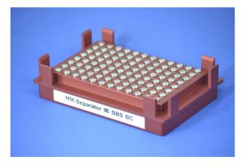
The magnetic separator is designed for U- and V-bottom microplates. It is not recommended for flatbottom or PCR plates. For PCR plates, the use of MM-Separator 96 PCR (Art.No. MDMG0005) is recommended. For DeepWell plates, the use of MM-Separator 96 DeepWell (Art.No. MDMG0013) is recommended. Contact magtivio for additional information and compatibility of microplates.
