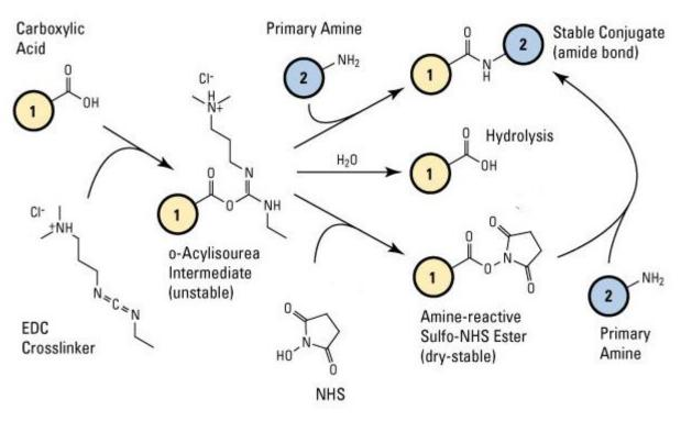
It is recommend to couple biomolecules via the 2-step method in order to prevent crosslinking effects.
